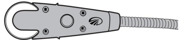
This side of the microphone should face **away** from you. The small 'cap' (larger disk in the middle) on the back is to access a Microphone gain adjustment.
